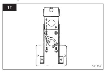
9.6 Feed the cable back through the hole as you replace the bracket. When the bracket is located correctly it will sit flush with the back panel without force required. If not positioned correctly the bracket will sit at an angle. See Diagram 18.
